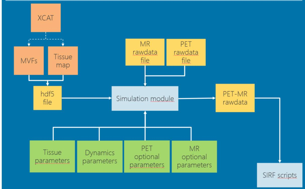
Fig. 1, Simulation framework design. The simulation module takes formatted hdf5 input containing the tissue segmentation and motion vector fields (MVFs). Based on MR and PET rawdata files the acquisition process is simulated. Additional variable parameters enable simulation customization beyond the ones defined in the rawdata files. The output is given in a standardized format and can be reconstructed using SIRF.
